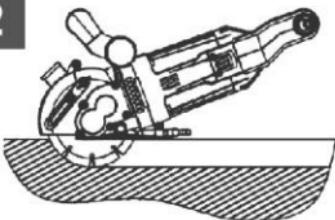
Cutting plane wall after wheel cover closing
