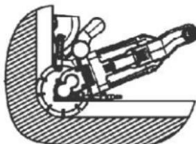
Cutting around the corner after opening wheel cover
